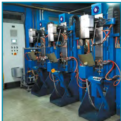
State of the art automatic welding and attaching machines are used for connecting the glass parts to each other.
