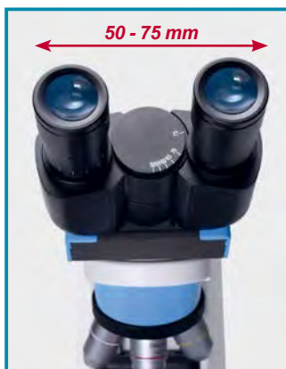
Featured with a 360° rotatable binocular head inclined at 30° with interpupillary distance adjustable 50 mm - 75 mm.
