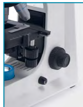
Coarse and fine adjustment is enabled with upper limit safety with 0,002 mm fine division and 20 mm maximum moving limit.
