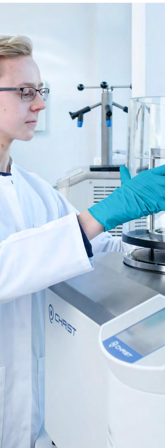
Freeze drying is not only used for water-based materials. Typical examples include HPLC fractions with organic or inorganic solvents, such as acetonitrile, TFA and other alcohols, or other products with t-butanol, DMSO, etc. The Alpha 3-4 LSCbasic is available in two defined packages, fully aligned to the requirements of freeze drying with solvents.
