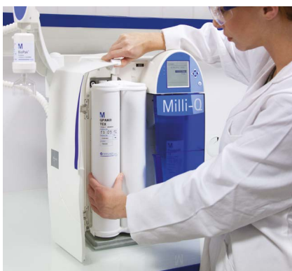
QPAK® polishing cartridge replacement
