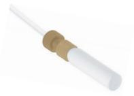
The No-Met polyethylene filter is designed for these applications, with inert polymeric fittings for 1/8" tubing and a 20 µm filter effectively eliminating metal contamination from the fluid path. Use them for IC and biochromatography applications.
