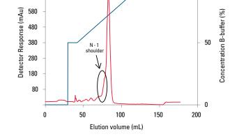
Resin: TSKgel SuperQ-5PW (20); Column size: 6.6 mm ID  $\times$  18.5 cm (6.3 mL); Mobile phase: A: 20 mmol/L NaOH; B: 20 mmol/L NaOH, 3.0 mol/L NaCl; Gradient: 50 % B (2 CV) 50-100 % B (15 CV), 100 % B (2 CV); Flow rate: 200 cm/h (1.14 mL/min); Detection: UV @ 254 nm; Sample load: 1.0 mg; Sample: crude phosphorothioate deoxyoligonucleotide
