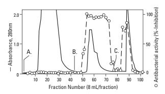
Column: TOYOPEARL Butyl-650S, 22 mm ID x 26 cm L Sample: crude protein from sea hare Aplysia kurodai; Mobile phase: multi-step  $(NH_4)_2SO_4$  in 50 mmol/L phosphate buffer (pH 7.0); A. load & wash: 40 % saturated  $(NH_4)_2SO_4$ ; B. 20 % saturated  $(NH_4)_2SO_4$ ; C. 0% saturated  $(NH_4)_2SO_4$ ; Detector: UV @ 280 nm
