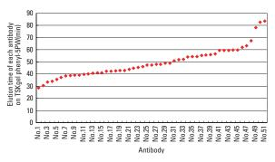
Plot of chromatographic elution times for 51 different mouse mAbs Column: TSKgel Phenyl-5PW; Mobile phase: (A) 0.1 mol/L phosphate buffer containing 1.8 mol/L ammonium sulfate (pH 7.0); (B) 0.1 mol/L phosphate buffer (pH 7.0);
