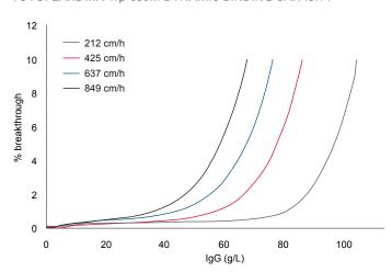
Column: TOYOPEARL MX-Trp-650M (6 mm ID x 4 cm); Sample: polyclonal human IgG (1 mg/mL) in 0.05 mol/L NaAc + 0.1 mol/L sodium chloride (pH 4.7); Linear velocity: 212, 425, 637, 849 cm/h; Detection: UV @ 280 nm
