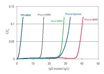
Column: 7.8 mm ID X 20 cm L; Sample: polyclonal human IgG Binding buffer: 1 g/L IgG in 0.8 mol/L (NH,) SO, + 0.1 mol/L sodium phosphate (pH 7.0); Linear velocity: 300 cm/h Temperature: 25 °C; Detector: UV @ 280 nm DBC was calculated at 10% of breakthrough.
