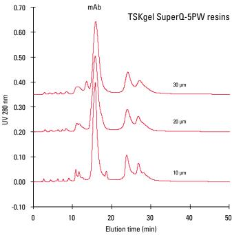
Resins: 1) TOYOPEARL SuperQ-650C (100 µm); 2) TOYOPEARL SuperQ-650M (65 μm); 3) TOYOPEARL SuperQ-650S (35 μm); 4) TSKgel SuperQ-5PW(30) (30  $\mu$ m); 5) TSKgel SuperQ-5PW(20) (20  $\mu$ m); 6) TSKgel SuperQ-5PW (10  $\mu$ m) Column size: 7.5 mm ID x 7.5 cm; Mobile phase: Buffer A: 0.02 mol/L Tris-HCI, pH 8.5; Buffer B: 0.5 mol/L NaCl in Buffer A;
