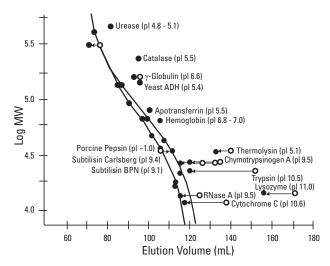
Column: TOYOPEARL HW-55F, 22 mm ID x 50 cm L; Elution: 25 mmol/L Tris-HCl with (•) or without (°) 0.5 mol/L NaCl, (pH 7.5); Flow rate: 16 cm/h; Temperature: 5 - 10 °C; Detection: UV @ 280 nm, 420 nm for heme proteins, 200 nm for proteins without aromatic amino acid
