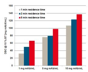
Column: TOYOPEARL AF-rProtein A HC-650F (6.6 mm ID  $\times$  2 cm L) Mobile phase: 100 mmol/L sodium phosphate pH 6.5; Residence time: 1, 2, 5 min; Detection: UV @ 280 nm Sample: monoclonal antibody mAbX @ 1, 5, 10 g/L in mobile phase DBC measured at 10 % breakthrough
