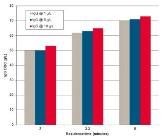
Column: TOYOPEARL AF-rProtein A HC-650F (5 mm ID  $\times$  5 cm L) Mobile phase: 20 mmol/L sodium phosphate, 150 mmol/L NaCl pH 7.4; Residence time: 2, 3.3, 5 min; Detection: UV @ 280 nm Sample: polyclonal human IgG @ 1, 5, 10 g/L in mobile phase DBC measured at 10 % breakthrough
