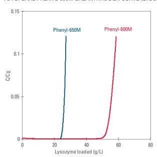
Binding capacity (g/L) (10% Breakthrough)
