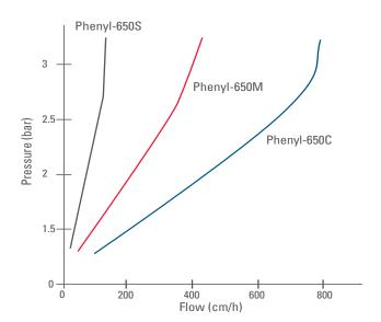
Column: TOYOPEARL Phenyl-650C, M and S, 25 mm ID x 25 cm L Mobile phase: 2 mol/L (NH<sub>4</sub>)<sub>2</sub>SO<sub>4</sub>
