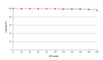
Column size: 5 mm ID  $\times$  5 cm L; Wash procedure: A: 20 mmol/L Na $_2 \rm{HPO}_4$  0.15 mol/L NaCl, pH 7.4 (10 CV)
