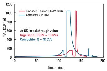
Column size: 6 mm ID x 40 mm L; Sample: polyclonal human IgG (1 mg/mL); Loading buffer: 15 mmol/LTris-HCl (pH= 8.7); Elution buffer: 15 mmol/L Tris-HCI (pH= 8.7) + 1.0 mol/L NaCI;
