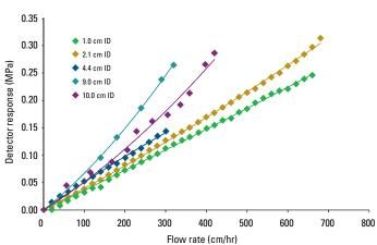
Column size: 1.0 cm ID, 2.1 cm ID, 4.4 cm ID, 9.0 cm ID, 10.0 cm ID; 20 cm normalized bed height; Mobile phase: DI  $\rm H_2O$
