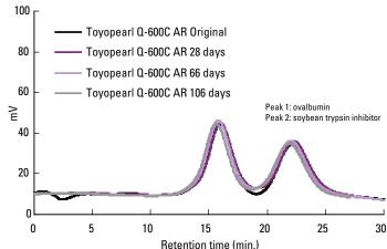
Column: 6.0 mm ID x 4 cm L; Flow rate: 1.0 mL/min; Elution: Buffer A: 0.05 mol/L Tris-HCl buffer (pH= 8.5); Buffer B: 0.05 mol/L Tris-HCl buffer + 1.0 mol/L NaCl (pH= 8.5); Gradient: 60-min linear gradient from buffer A to buffer B; Detection: UV @ 280 nm
