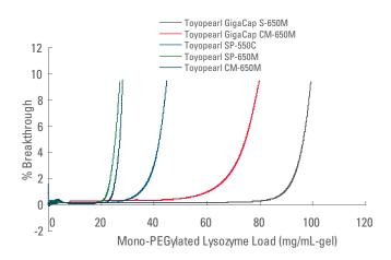
Dynamic binding capacities were determined at 10% breakthrough Column size: 6 mm ID x 40 mm L; Sample: mono-PEGylated lysozyme; Loading buffer: 20 mmol/L phosphate buffer (pH= 7.0) Elution buffer: 20 mmol/L phosphate buffer (pH= 7.0) + 0.5 mol/L NaCl Linear velocity: 212 cm/h; Detection: UV @ 280 nm PEG MW= 5kDa
