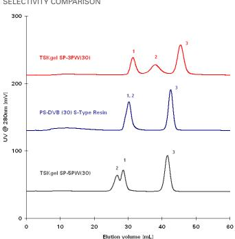
Column: 7.5 mm ID x 7.5 cm L; Mobile phase: A: 20 mM sodium citrate buffer (pH 3.2)/ethanol = 8/2 (v/v); B: 1.0 mol/L NaCl in 20 mM sodium citrate buffer (pH 3.2)/ethanol = 8/2 (v/v); Gradient: 60 min linear gradient from Buffer A to Buffer B; Flow rate: 1.0 mL/min;
