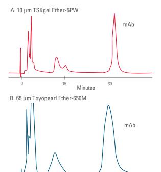
Column: A. TSKgel Ether-5PW, 7.5 mm ID  $\times$  7.5 cm L B. TOYOPEARL Ether-650M, 7.5 mm ID  $\times$  7.5 cm L Sample: anti-chicken 14 kDa lectin, diluted ascites fluid, A. 1.5 mg in 100  $\mu$ L; B. 0.76 mg in 50  $\mu$ L
