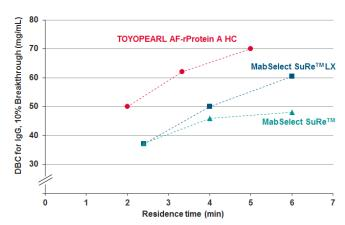
Mobile phase: 20 mmol/L sodium phosphate, 150 mmol/L NaCl pH 7.4; Residence time: 2, 3.3, 5 min; Detection: UV @ 280 nm; Sample: polyclonal human IgG @ 1 g/L in mobile phase; DBC measured at 10 % breakthrough. MabSelect SuRe™ and MabSelect SuRe™ LX DBC data from GE brochure. MabSelect SuRe™ and MabSelect SuRe™ LX are registered trademarks of GE Healthcare Bio-Sciences AB,
