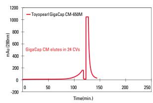
Column size: 6 mm ID x 40 mm L; Sample: polyclonal human IgG (1 mg/mL); Loading buffer: 50 mmol/L sodium acetate buffer (pH= 4.7); Elution buffer: 15 mmol/L Tris-HCl (pH= 8.7) + 1.0 mol/L NaCl Linear velocity: 212 cm/h; Detection: UV @ 280 nm
