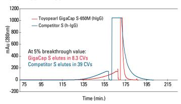
Column size: 6 mm ID x 40 mm bed; Sample: polyclonal human IgG (1 mg/mL); Loading Buffer: 0.1 mol/L acetate buffer (pH= 4.7) Elution Buffer: 0.1 mol/L acetate buffer (pH= 4.7) + 1.0 mol/L NaCl Linear velocity: 212 cm/h; Detection: UV @ 280 nm
