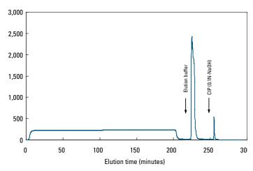
Resin: TOYOPEARL Protein A; Column size: 5 mm ID  $\times$  5.0 cm L; Mobile phase: Buffer A: 20 mmol/L sodium phosphate containing 0.15 mol/L NaCl, pH 7.4, Buffer B: 0.1 mol/L citrate, pH 3.0; Flow rate: 61 cm/h (0.2 mL/min); Residence time: 5 min; Sample: 40 mL of CHO cell culture, containing 1.0 g/L humanized IgG,
