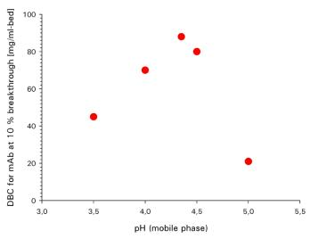
Column size: 6.6 mm ID x 2.2 cm; Binding buffer: 0.1 mol/L acetate buffer (pH 3.5 - 5.0) + 0.2 mol/L NaCl; Linear velocity: 150 cm/h; Detection: UV @ 280 nm; Sample: humanized monoclonal IgG Dynamic binding capacity (DBC) calculated at 10 % breakthrough.
