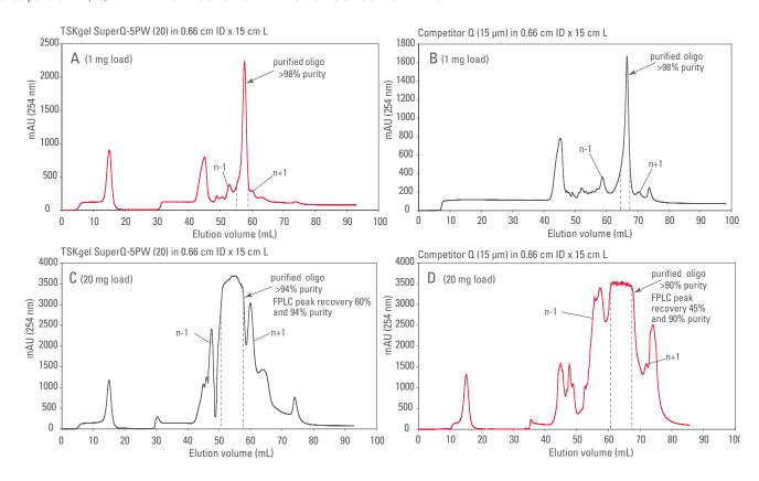
Column: 0.66 cm x 15 cm L (5.1 mL) (resin as noted in figure); Flow rate: 1.43 mL/min (250 cm/h)  $\,$
