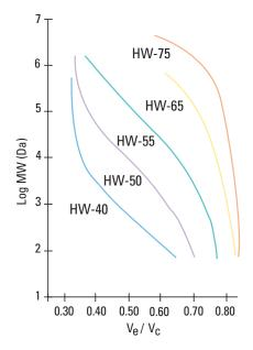
Column: 22 mm ID x 30 cm L; Sample: Protein standards; Mobile phase: 0.06 mol/L phosphate buffer (pH 7.0) in 0.06 mol/L KCI; Legend: Ve = elution volume, Vc = column volume; Detection: UV @ 280 nm
