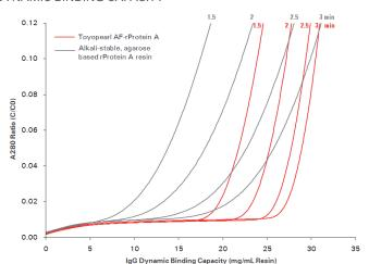
Breakthrough curves for h-lgG loading (polyclonal, 10 g/L) Typical DBC at 10 % breakthrough: 30,5 g/L @ 100 cm/h (3 min residence time) - 24 g/L @ 200 cm/h (1.5 min residence time); Column: 5 mm ID x 5 cm L; Mobile phase: 20 mmol/L sodium phosphate buffer pH 7.2 containing 150 mmol/L NaCl; Sample conc.: 10 g/L; Residence time: 1.5, 2.0, 2.5, 3.0 min
