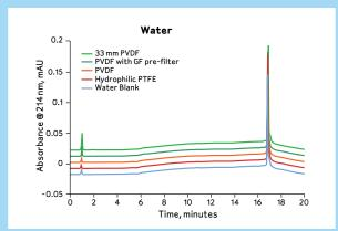
Low water extractables indicate that Millex filters are ideal for dissolution studies and other aqueous-based sample prep protocols.
