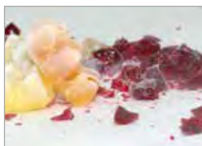
Material embrittled with liquid nitrogen
