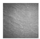
Electroformed nickel (EFNi)
