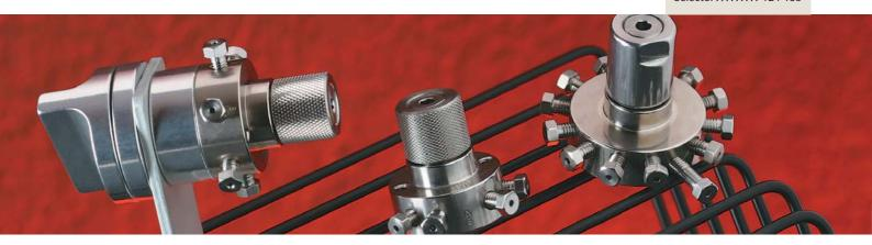
The standard valve body material is Nitronic 60, a gall-resistant stainless steel which has proven superior to Type 316 or 303 in the majority of applications. Valves may also be ordered in Hastelloy C-22, Inconel 600, Type 316 stainless, Monel 400, Nickel 200, Nitronic 50, or Titanium.
