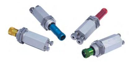
Flow controllers provide a stable flow rate under varying pressure. VICI flow controllers are precision machined from aluminum or stainless bar stock to eliminate the contamination often found in die cast parts. Positive flow
