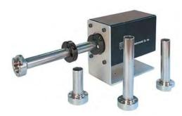
Valves which will be installed in ovens or heated zones require a standoff assembly, which locates the actuator out of the heated zone and supports both the valve and the handle or actuator. The 5/8" outside diameter standoff tube extends through the oven wall and is secured by means of a clamp ring supplied with the assembly.
