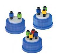
The VICI cap is the most economical way to helium sparge and deliver HPLC mobile phases. The insert is manufactured from PTFE, with a polypropylene screw cap and an EPDM\* O-ring which is resistant to commonly used HPLC solvents.
