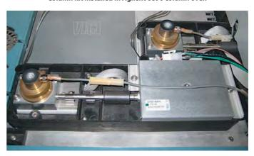
View of relocated Agilent FID to permit use of fast GC column kit
