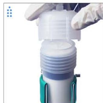
Put back the screw cap onto the cartridge.
