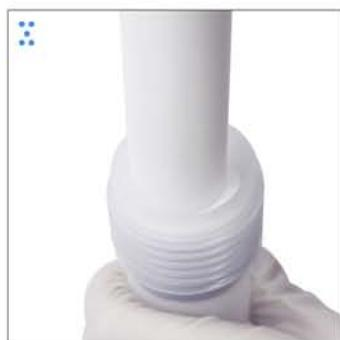
Use the frit insertion rod to press the frit into space.
