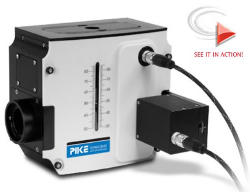
AutoPRO Software (left) configured for the Automated VeeMAX III (shown above with polarizer option) for automated depth profiling studies.
