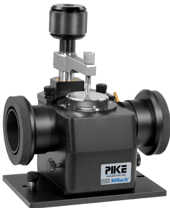
MIRacle – Highest IR Throughput ATR.
