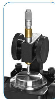
MIRacle Micrometer Clamp – for low pressure applications
