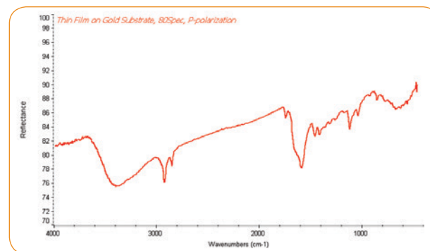
FTIR spectrum of an ultra-thin film on a reflective substrate using p-polarized IR beam.
