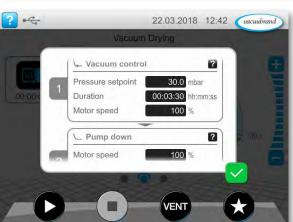
VACUU·SELECT includes predefined vacuum procedures for all common lab applications. The process steps and control parameters can easily be adjusted to suit any application.
