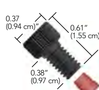
P-945x 2 Delrin Nut, M6 with P-940 Ferrule
