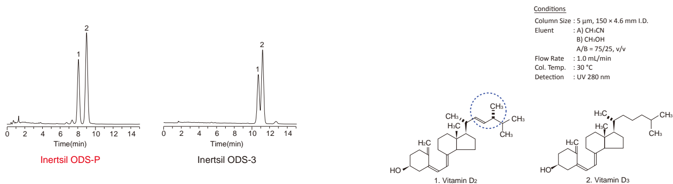
Figure 2 : Comparison of Selectivity Between a Polymeric and Monomeric Type C18 Phase
