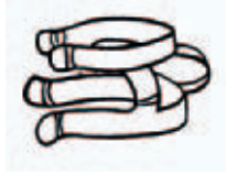
SPRING STEEL CLIPS, KECK FOR CONICAL JOINTS
