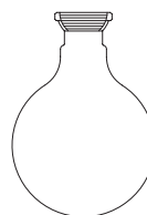
ROUND BOTTOM FLASKS, ONE NECK neck with spherical ground cup
