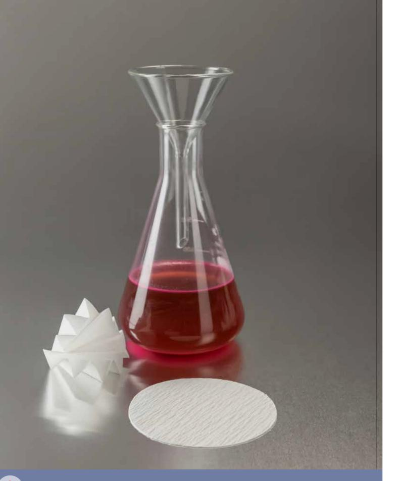
Creped filter papers have a particularly large surface area and correspondingly shorter filtration times.
