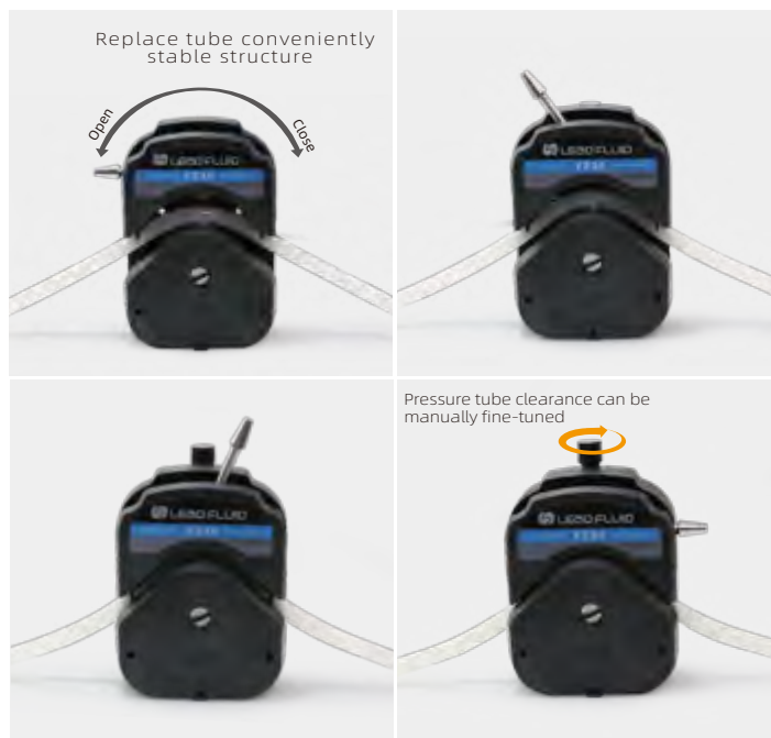
Installation tube method
