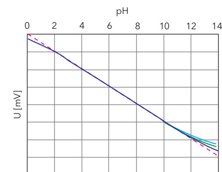
6 Exemplary mV curve of various electrode for different pH values.
